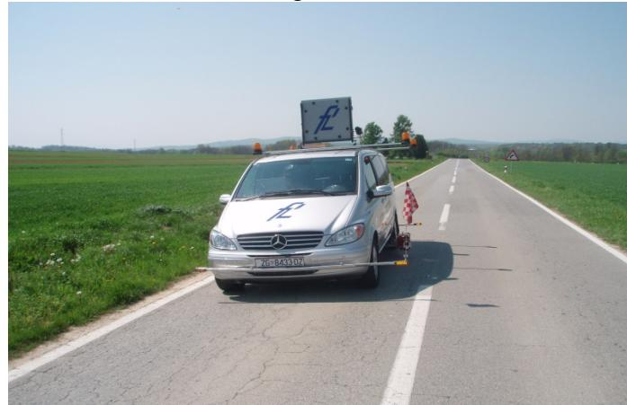
**Figure 7.** Measurement vehicle with dynamic retroreflectometer
