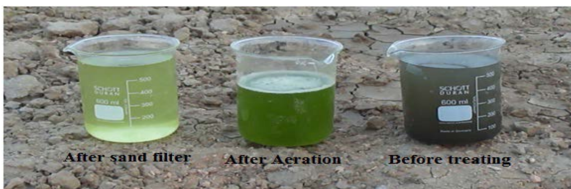
Plate (10) Picture show the difference in color without and with using sand filter.
