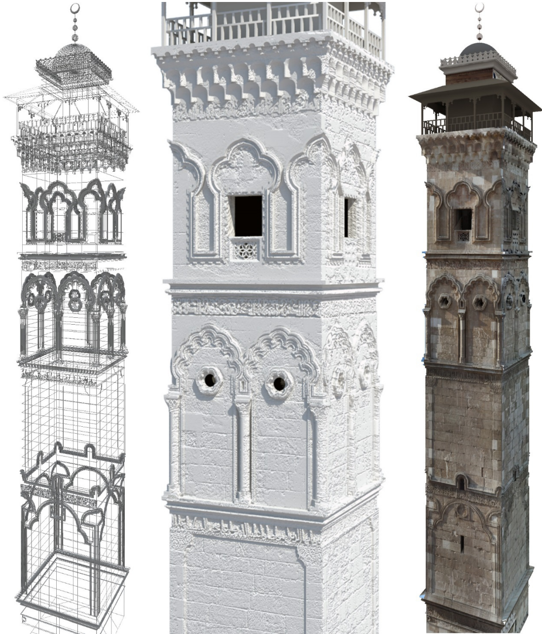
6/ The wireframe, shaded and textured model
