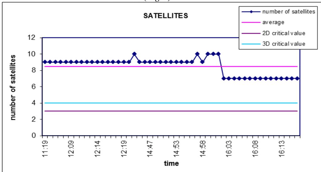
Fig.3: Number of satellites during GPS measurement (11.09.2013).
