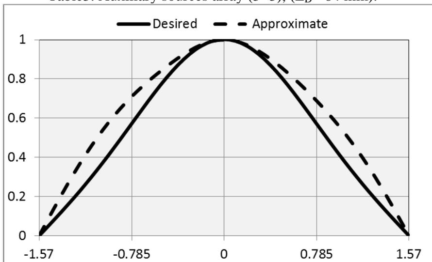
Fig. 4. Amplitude radiation pattern for the undisturbed internal sources  $F_{oi}(\theta, \varphi)$  and the approximate with the auxiliary sources table3.
