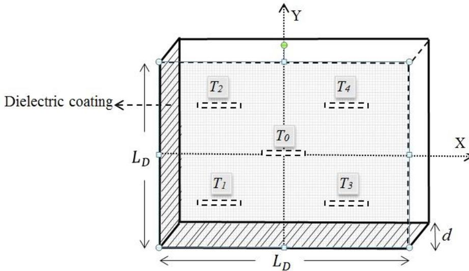
Fig. 5. Slot emitters array under a dielectric coating.
