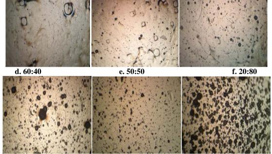
Fig 2.2: Crystallinity of Medium Molecular Weight Chitosan-PCL Film
