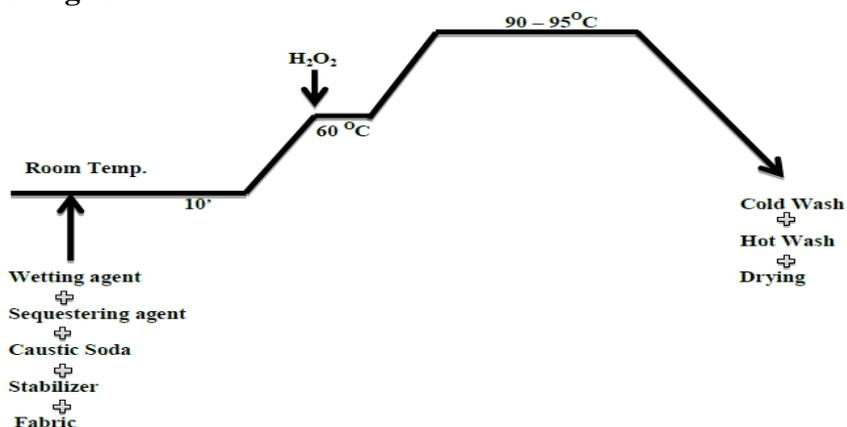
Figure-1: Process diagram of combined Scouring & Bleaching
