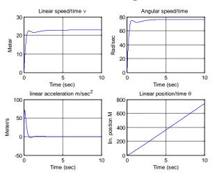
**Figure 5(b)** linear speed/time, angular speed time response curves, feeding back load toque to both motor as load torque and as equivalent voltage control system
