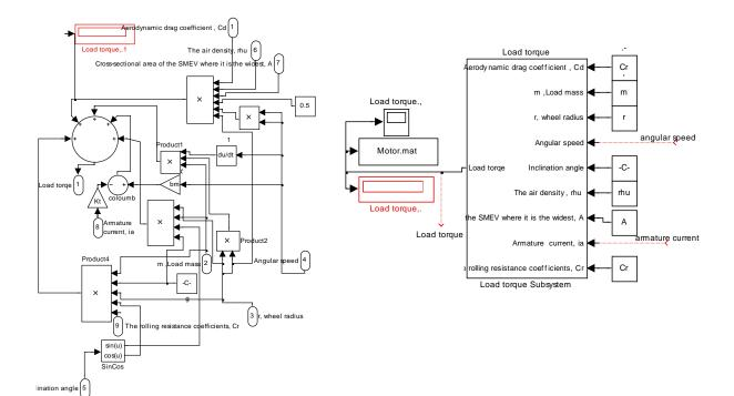
Figure 2(a) EV Disturbance torque and function model
