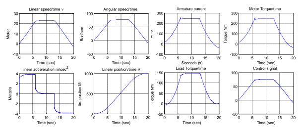
**Figure 7(b)** EV closed loop linear speed/time, angular speed /time, linear acceleration /time, current/time, control signal//time, motor torque/time response curves for reference motion profile input applying two PID controller for both loops .
