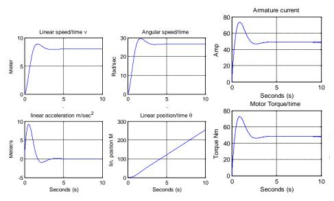
Figure 3(d) EV open loop step response curves; linear speed/, angular speed /time, linear acceleration /time, current/time, motor torque/time
