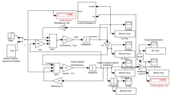
Figure 3(b) simulink model based on state space equations Reference motion profile Reference training Refere
