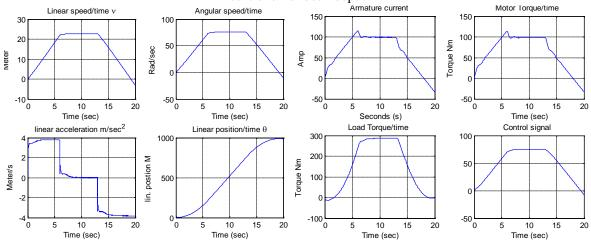
**Figure 7(c)** EV closed loop linear speed/time, angular speed /time, linear acceleration /time, current/time, control signal//time, motor torque/time response curves for reference motion profile input applying two PID controller for both loops applying proposed design *relating load torque*, *tachometer and corresponding*
