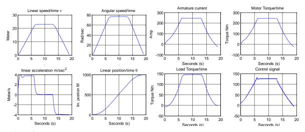
**Figure 4(b)** EV closed loop linear speed/time, angular speed /time, linear acceleration /time, current/time, control signal//time, motor torque/time response curves for reference motion profile input applying one control loop with PID
