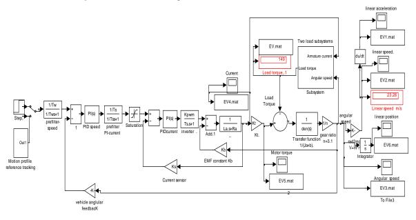
Figure 8(b)Two PI controller with two prefilter
