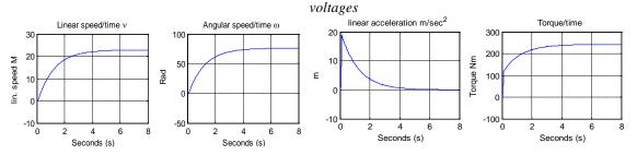
**Figure 7(d)**Linear speed/time, angular speed/time Linear acceleration/time, torque/time, response curves of EV for desired output linear speed of 23 m/s (that is 82.8 km/h), applying PI controller for both , inner and outer, loop
