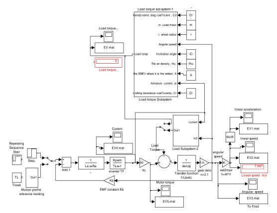
Figure 3(a) Basic EV open loop simulink model, dynamics is coupled with the wheel rotational velocity via characteristics of the electric motor and surface; two disturbance models are included with manual switch.
