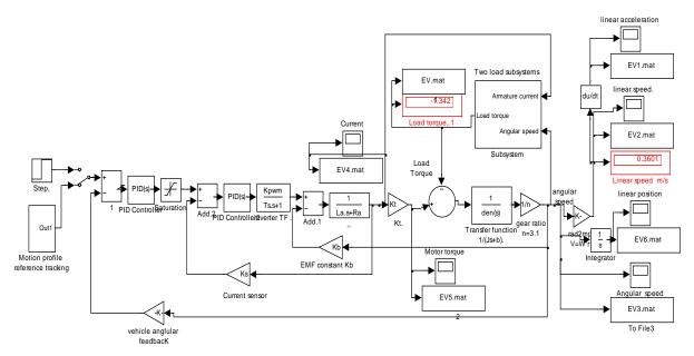
Figure 8(a) two control loops model, inner current with current sensor
