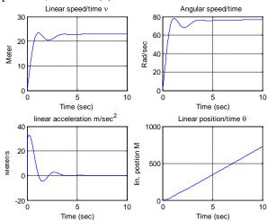
Figure 5(c) linear speed/time, angular speed time response curves, feeding back load toque as equivalent voltage *just* to control system
