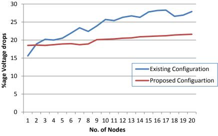
Figure 3 voltage drops before and after the proposed reconfiguration
