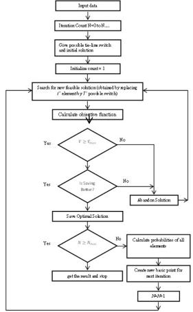
Figure 1 Flow Chart for network reconfiguration under proposed algorithm
