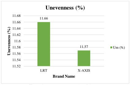
Figure 1: Unevenness properties of the yarn
