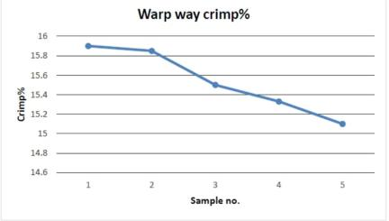
Figure 4: Effect of warp tension on warp yarn crimp%
