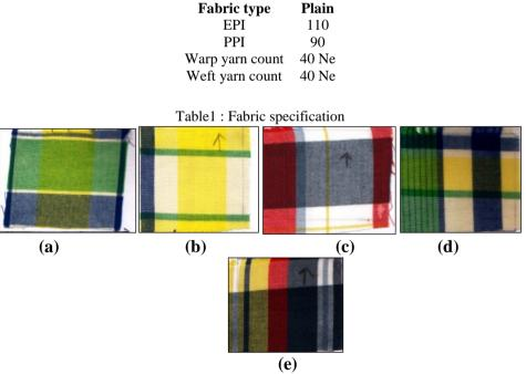
Figure 3: Woven fabric produced at different warp tension a) 2100N b) 2150N c) 2200N d) 2250N e) 2300N
