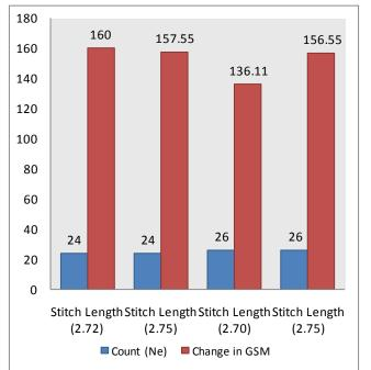
Figure 3.2 Changes in GSM with changes in stitch length and yarn count
