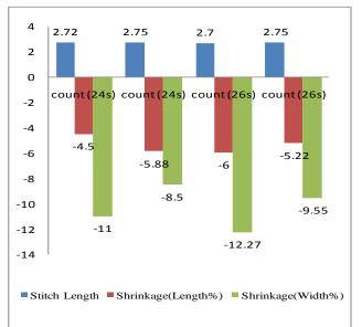
Figure 3.1 Changes in Shrinkage percentage with changes in count and stitch length
