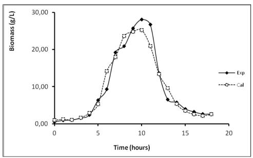
Figure 6: Comparison of experimental (exp) and predicted (cal) biomass evolution during the time of batch fermentation
