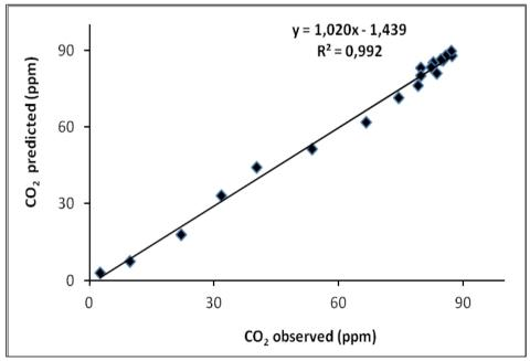
Figure 12: Regression curve between predicted and observed values for CO<sub>2</sub>
