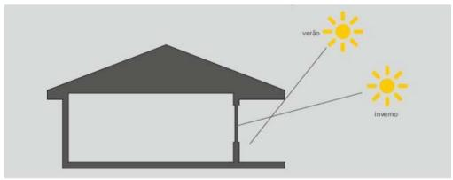
summer, when the sun is placed on a higher position, also contributes to the minimization of solar gains and, therefore, the building's cooling needs.
