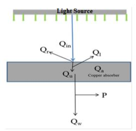
Figure. 1. Schematic diagram of the energy flow of the system shown in Fig. 1.
