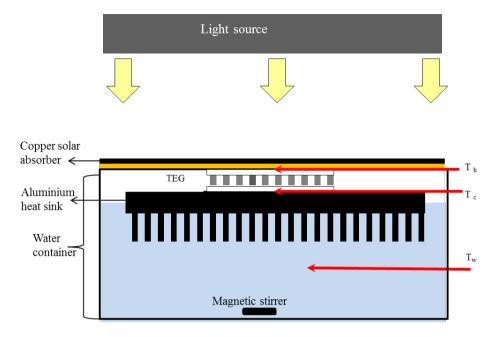
Figure. 1. System design and construction
