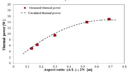
Figure 5. The measured and the calculated results of the heat power as function of the aspect ratio.
