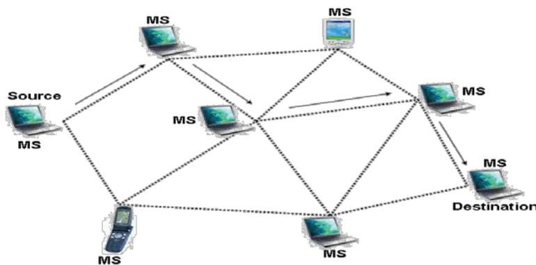
**Figure 2. Diagram of a MANET topology**
