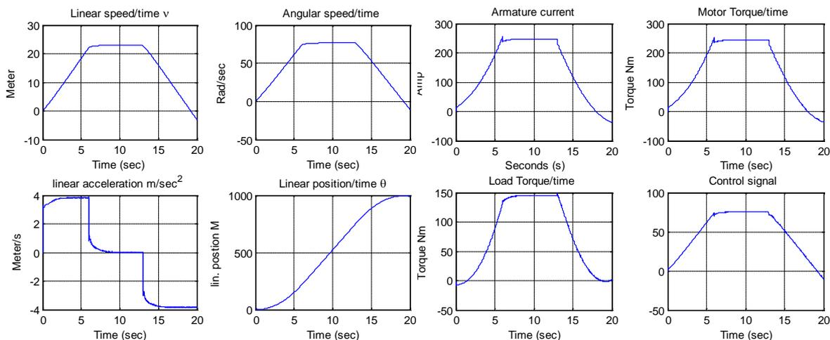
**Figure 7(b)** EV closed loop linear speed/time, angular speed /time, linear acceleration /time, current/time, control signal//time, motor torque/time response curves for reference motion profile input applying two PID controller for both loops .
