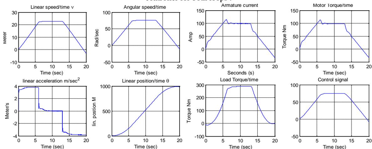
**Figure 7(c)** EV closed loop linear speed/time, angular speed /time, linear acceleration /time, current/time, control signal//time, motor torque/time response curves for reference motion profile input applying two PID controller for both loops applying proposed design relating load torque , tachometer and corresponding voltages
