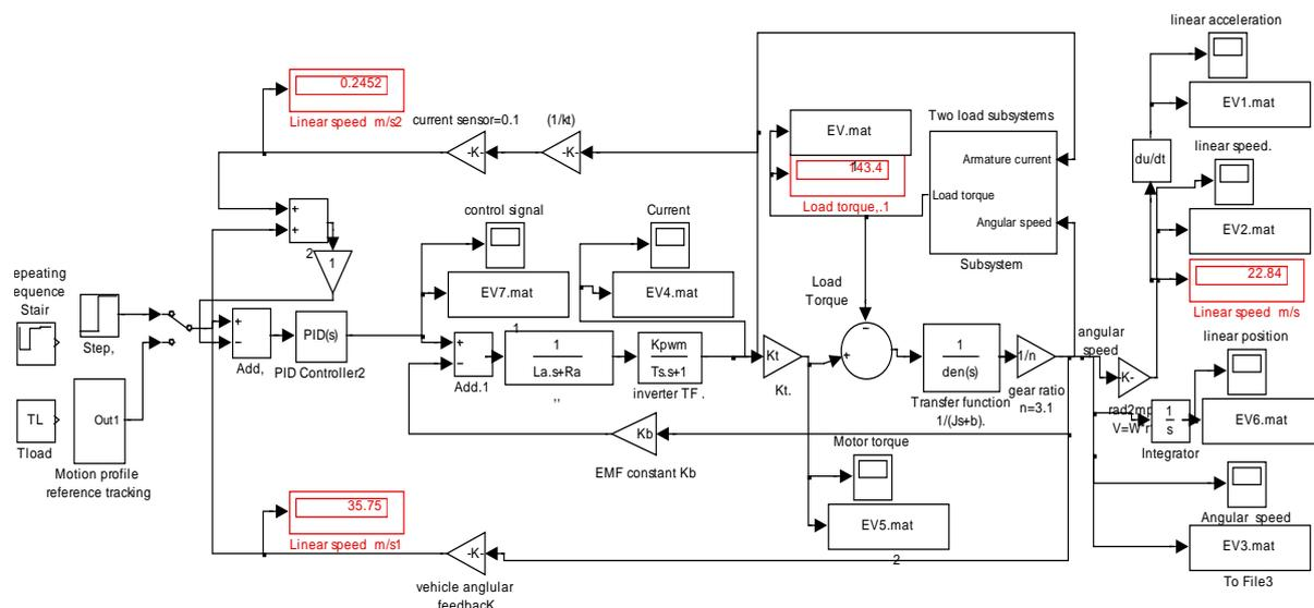
Figure 5(a) One closed loop control; Structure (2)
