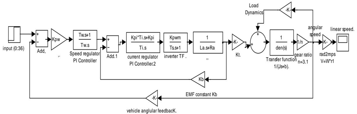
Figure SMEV model inner current and outer speed loops.
