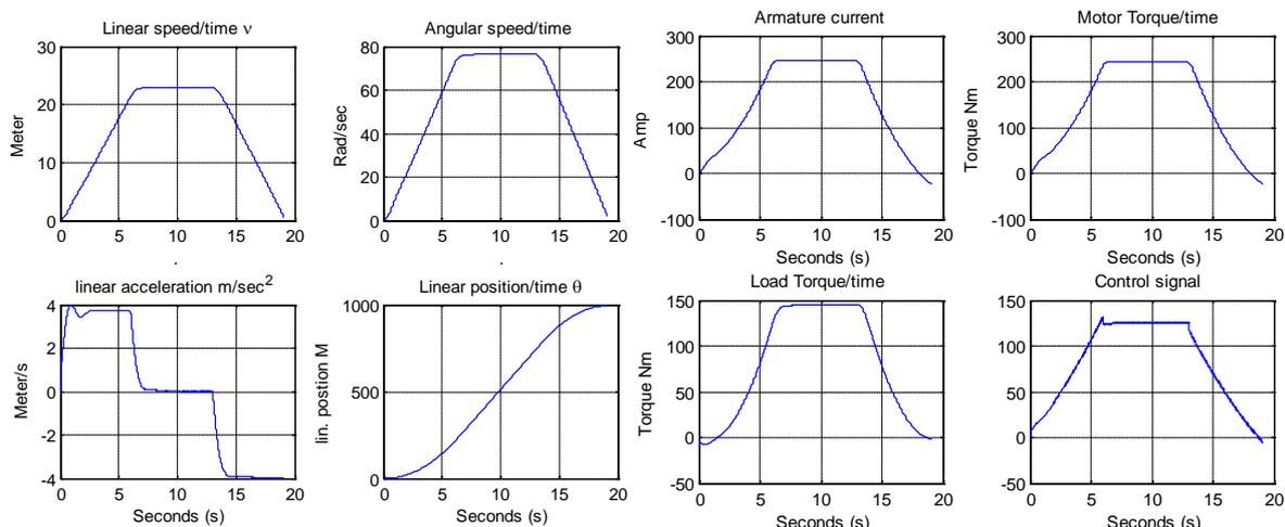
**Figure 4(b)** EV closed loop linear speed/time, angular speed /time, linear acceleration /time, current/time, control signal//time, motor torque/time response curves for reference motion profile input applying one control loop with PID
