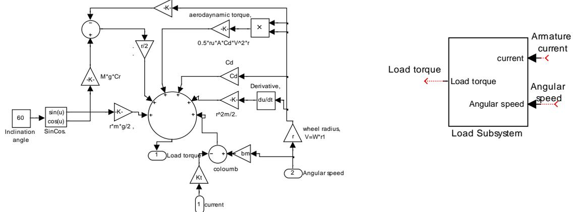
Figure 2(b) EV Disturbance torque and function model
