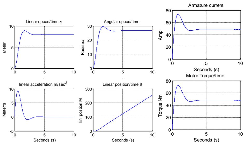
**Figure 3(d)** EV open loop step response curves; linear speed/, angular speed /time, linear acceleration /time, current/time, motor torque/time
