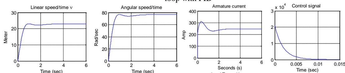
**Figure 4(c)** EV closed loop linear speed/time, angular speed /time, current/time, control signal//time, response curves for step input applying one control loop with PID
