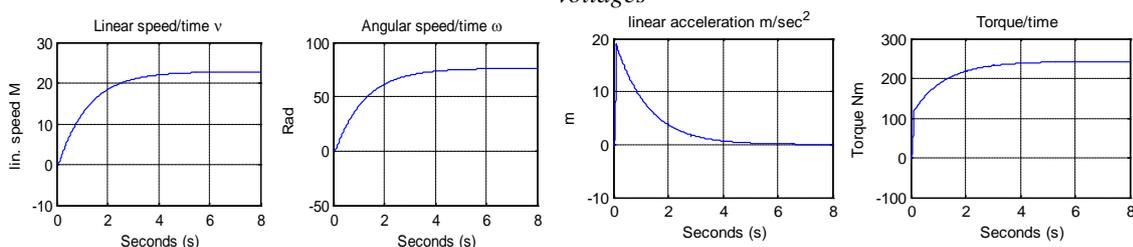
**Figure 7(d)**Linear speed/time, angular speed/time Linear acceleration/time, torque/time, response curves of EV for desired output linear speed of 23 m/s (that is 82.8 km/h), applying PI controller for both , inner and outer, loop
