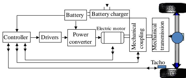
**Figure 1** Architecture, Major components of electric vehicle (Farhan A. Salem, 2013)
