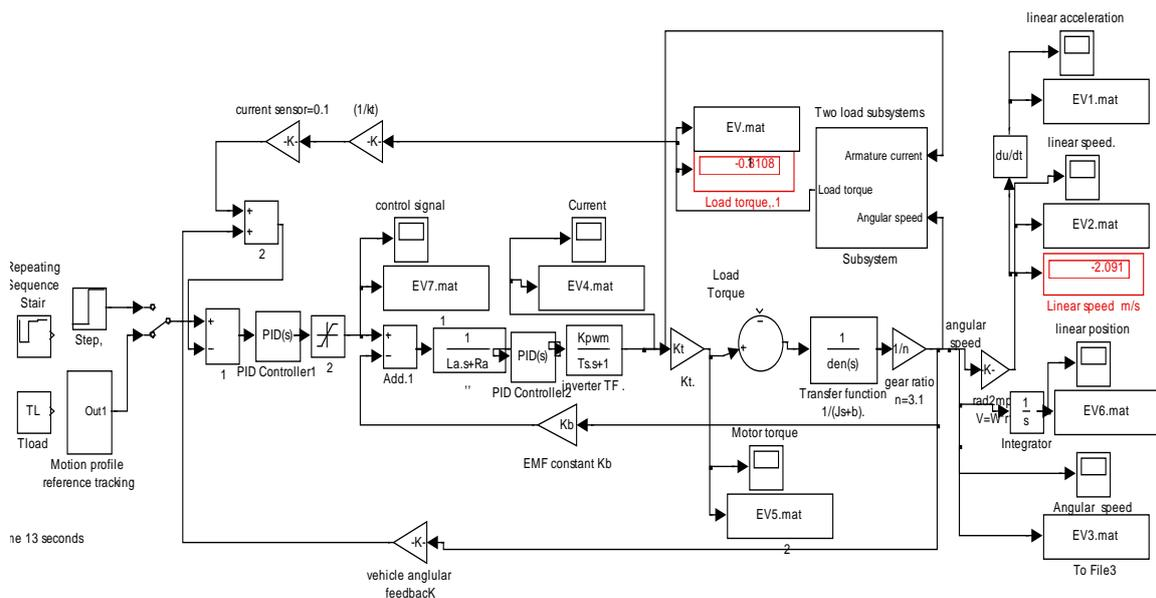
Figure 7(a) block diagram applying two controllers inner and outer,(PI, or PID)
