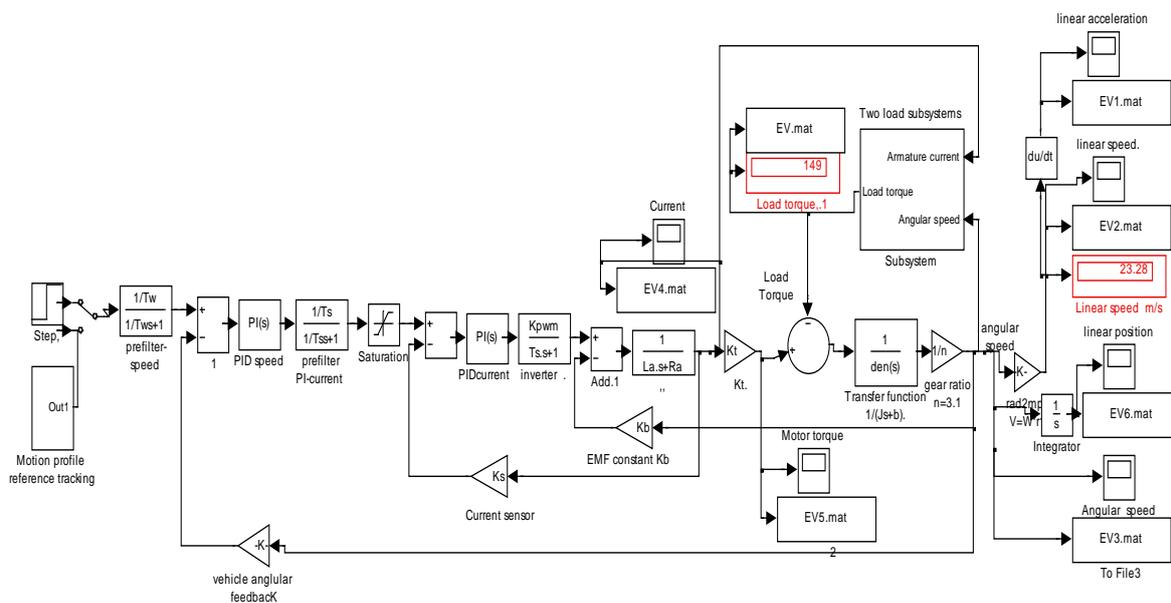
**Figure 8(b)** Two PI controller with two prefilter
