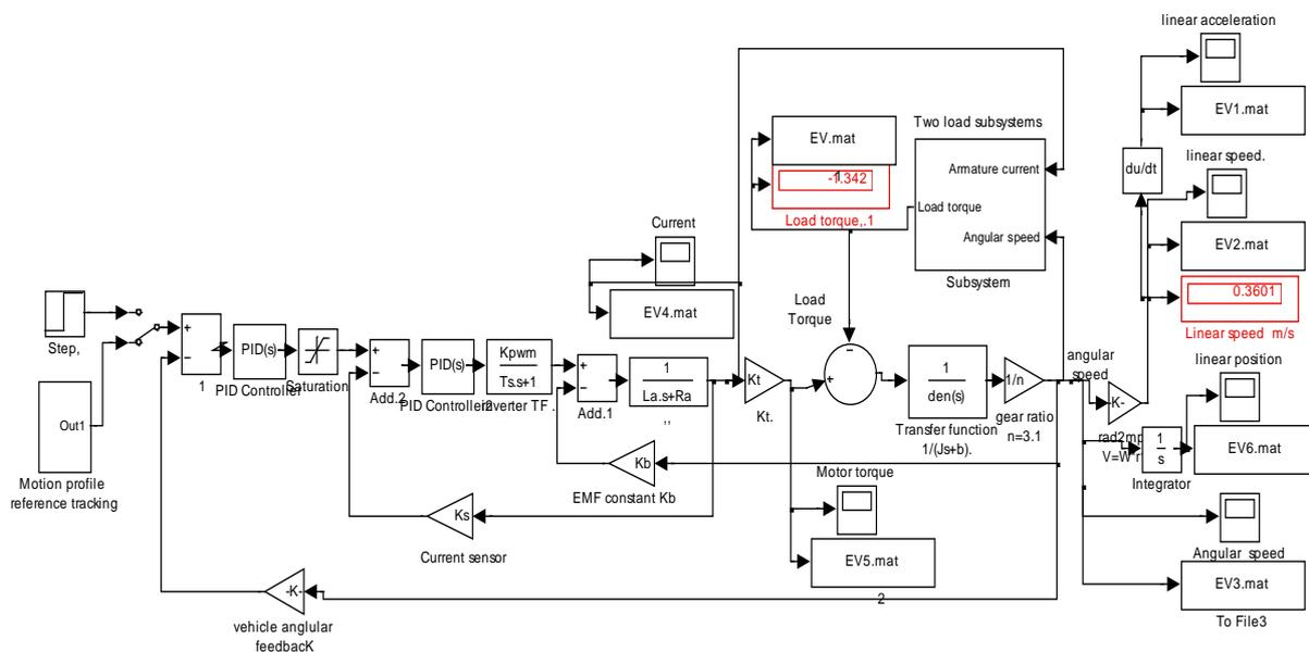
**Figure 8(a)** two control loops model, inner current with current sensor
