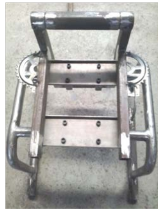
Figure 8. Shoulder CPM Chair during Fabrication.
