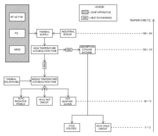
Fig.7 – "Hot" and "Cold" thermal supplies
