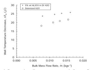
Figure 9. Decrease in wall temperature versus bulk mass flow rate.
