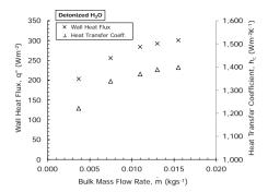
Figure 7. Wall heat flux versus mass flow rate (5% wt  $AL_2O_3$ ).
