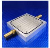
Figure 1a. Experimental setup of the electronic heat sink system.
