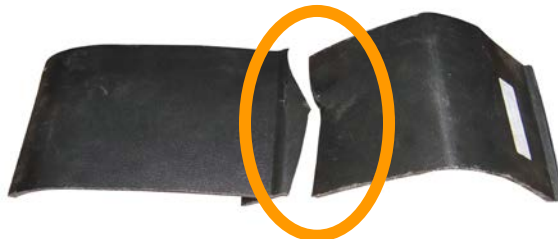
Fig. 10 Broken specimen (tested with filling material -sponge 30 in intensity)
