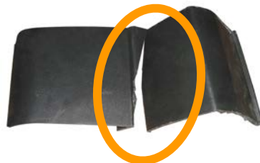
Fig. 10 Broken specimen (tested with filling material -sponge 30 in intensity)
