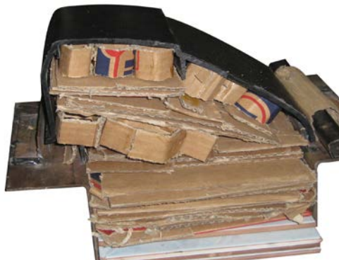
Fig. 7 Double layers of honey comb cardboard cells and cardboard sheets
