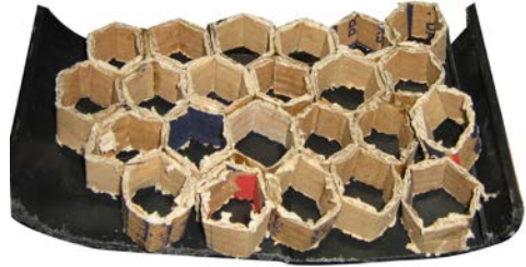
b. specimen with honey comb cell of cardboard
