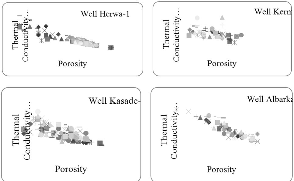
Fig. 6: Thermal conductivity-porosity profiles for Wells Herwa-1, Kerma-1, Kasade-1, and Albarka-1
