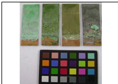
Figure 10: From left, corroded 5% tin bronze without inhibitor, corroded and treated with BTA, salicylaldoxime and cysteine after the high relative humidity and temperature experiment
