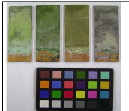
Figure 4: From left, corroded 5% tin bronze without inhibitor, corroded and treated with BTA, salicylaldoxime, and cysteine
