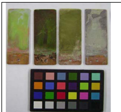
Figure 3: From left, corroded copper without inhibitor, corroded and treated with BTA, salicylaldoxime and cysteine
