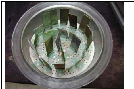
Figure 2: The set-up of the coupons in the desiccator for the high relative humidity and temperature experiment
