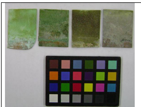
Figure 5: From left, corroded 12% tin bronze without inhibitor, corroded and treated with BTA, salicylaldoxime, and cysteine
