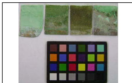
Figure 11: From left, corroded 12% tin bronze without inhibitor, corroded and treated with BTA, salicylaldoxime, and cysteine after the high humidity and temperature experiment
