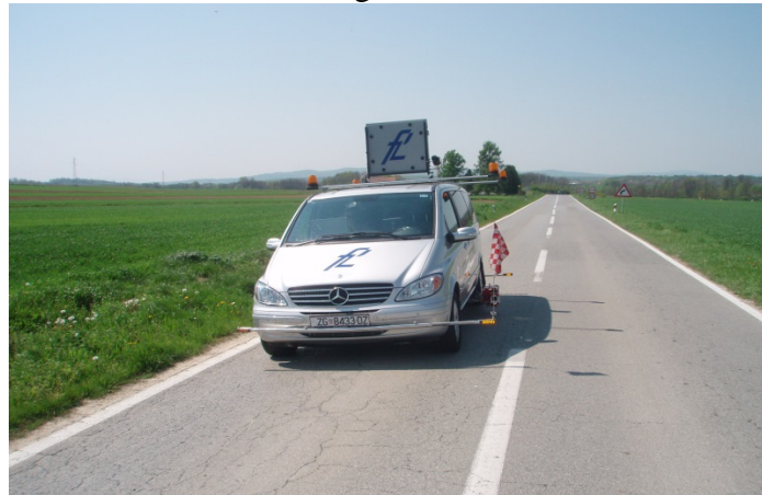
Figure 7. Measurement vehicle with dynamic retroreflectometer Source: Prepared by the authors
