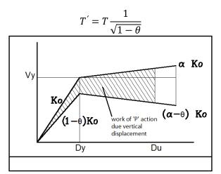
For the possible values of the coefficient of stability that extends from 0 to 0.2 increase in the period of free vibrations is not very significant in terms of design. However, in view of the study of  $P-\Delta$  effect has a significant impact. Comparisons are made between the behavior of response spectrum, and as well as land tremblings are invariable in nature , a small change in period, brings itself to be a difference between the two analysis evaluated.
