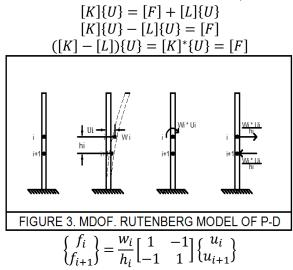
{F}- lateral forces ; [L]- factor matrixes 'Wi/hi' of th P- $\Delta$  momentums ; [K]\* - linear matrix of the system including P- $\Delta$ . [K]- linear matrix of the system excluding P- $\Delta$ ; {U}-lateral displacements.
