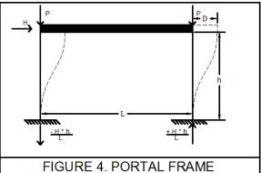
This distribution of the moment to the beam and vice versa will retain the same proportion, whether this moment will arise from the lateral loads or it comes from the P -  $\Delta$  effect. Any internal force that arises in the structure arises as a backlash of external action, with the same size regardless of what would be the nature of this action.
