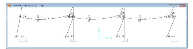
FIGURE 10. DIAGRAM OF MOMENTS FROM QUAKE ANALYSIS : 413.45 ; 484.53 ; 490.75 ; 498.41
