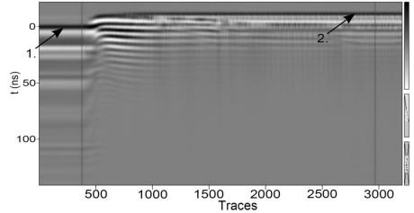
**Figure 3.** In experiment obtained GPR profile. 1. – identified direct signal when GPR antenna is on ground (corresponds to figure 2A). 2. – identified direct signal when GPR antenna is lifted in the air (corresponds to figure 2B).
