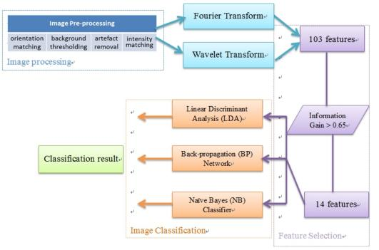
Fig. 2.1 – Block diagram of complete image classification system
