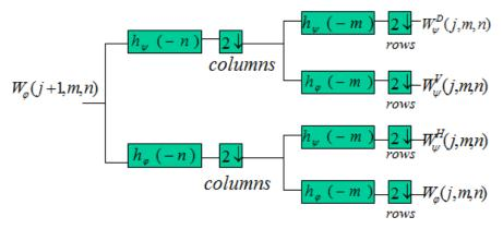
Fig. 1.1. Fast 2D wavelet transform (algorithm flow chart retrieved from the course note of Digital Image Processing in Memorial University)
