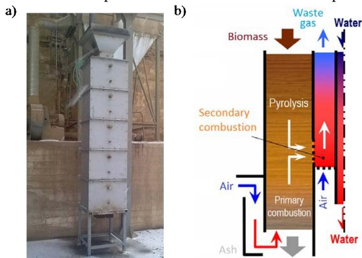
Fig. 2 Three-stage furnace: a) experimental furnace, b) functional scheme
