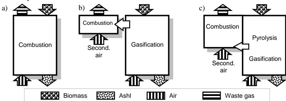
Fig. 1 Types of burning process: a) single-stage, b) two-stage, c) three-stage
