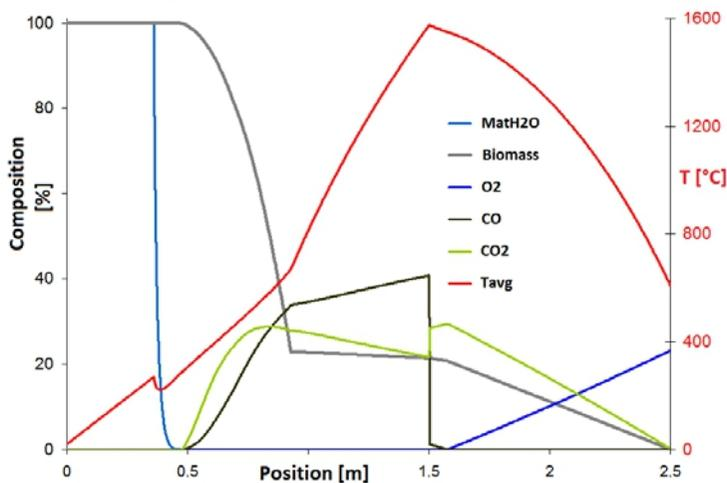
Fig. 8 Results of the simulations for alternative 2 – production of „Syngas“
