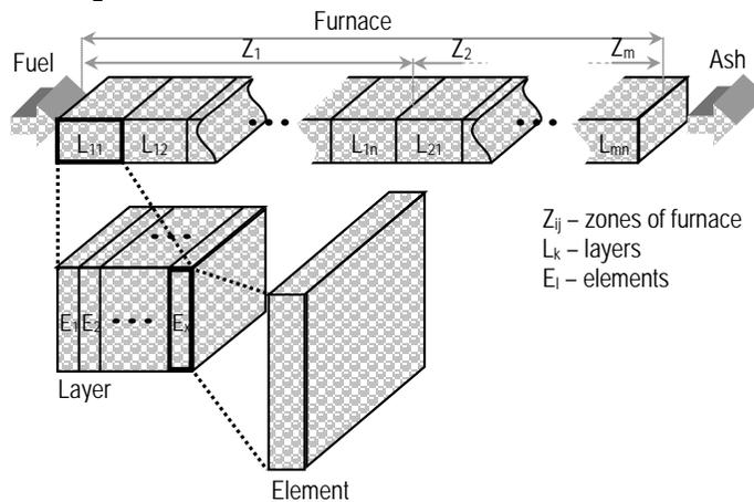
Fig. 3 Furnace decomposition
