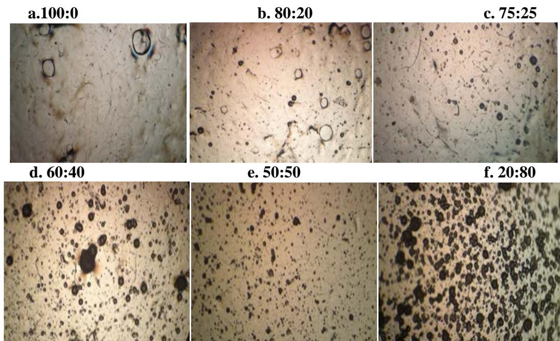
Fig 2.2: Crystallinity of Medium Molecular Weight Chitosan-PCL Film
