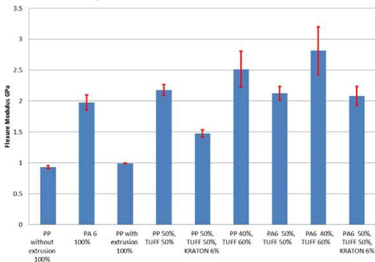
Figure 2 Flexural strength measurements
