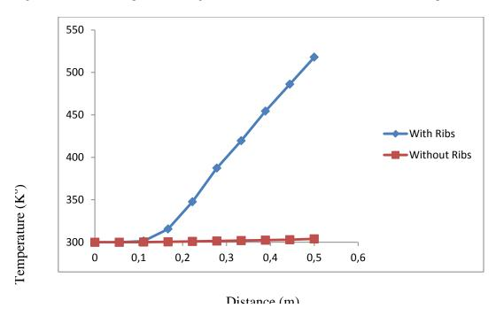
Fig. (9) Variation of Temperature Along the Center line of Tube at Constant Surface Temperature (1200 K°)
