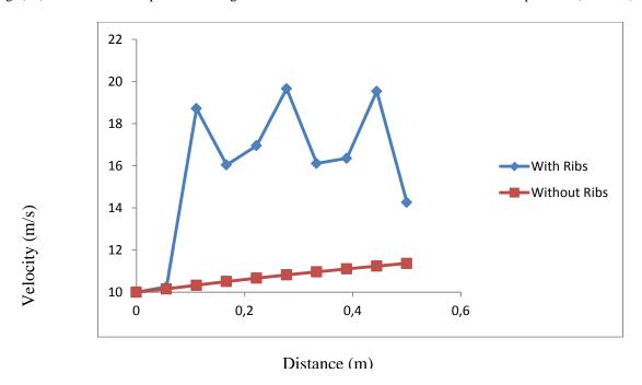
Fig. (11) Variation of Velocity Along the Center line of Tube at Constant Surface Temperature (1000 K°)
