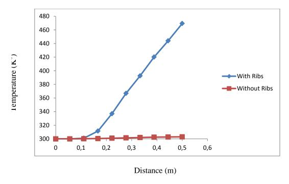
Fig. (8) Variation of Temperature Along the Center line of Tube at Constant Surface Temperature (1000 K°)
