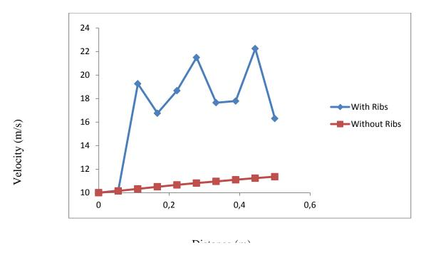
Fig. (13) Variation of Velocity Along the Center line of Tube at Constant Surface Temperature (1400 K°)
