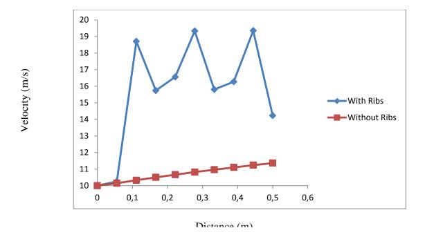
Fig. (12) Variation of Velocity Along the Center line of Tube at Constant Surface Temperature (1200 K°)
