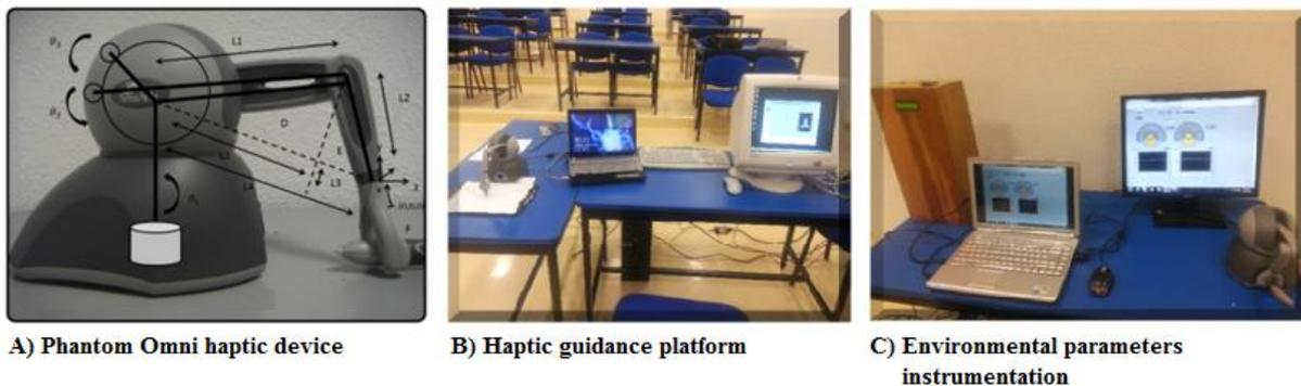
The Figure 6.1 represents the experimental platform based on Omni Phantom haptic device (A), the defined task for haptic guidance (B), and the measurement of environmental parameters (C: temperature, humidity, lighting and noise).
