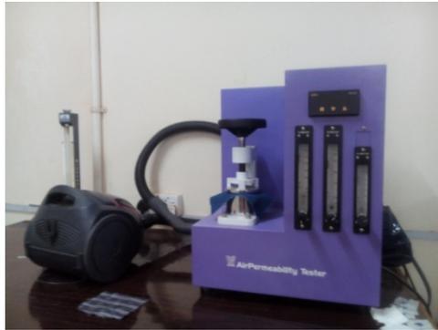
Figure 11. MAG Air Permeability Tester
