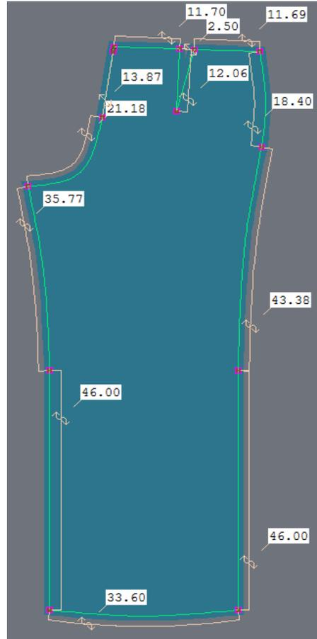
**Figure 16.** Drafted shape underside pattern piece with measurements.
