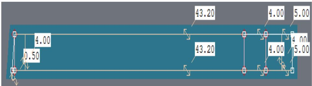
**Figure 14.** Drafted shape waistband pattern piece with measurements.
