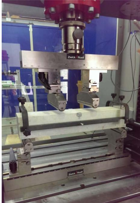
Fig. 4: Flexural Strength Test Setup for Beam Specimens
