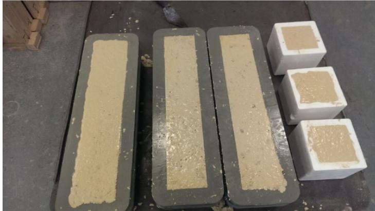
Fig. 2: Casting of SCC Cubes and Beams
