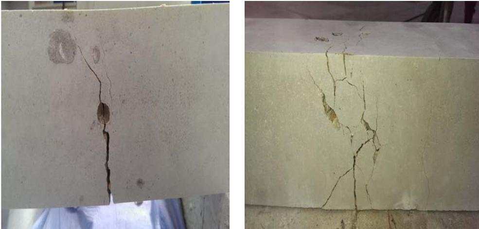
Fig. 7: Failure Mode and Crack Pattern of SCC Beams
