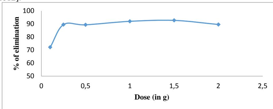
Figure 8: effect of adsorbent dosage on the adsorption.
