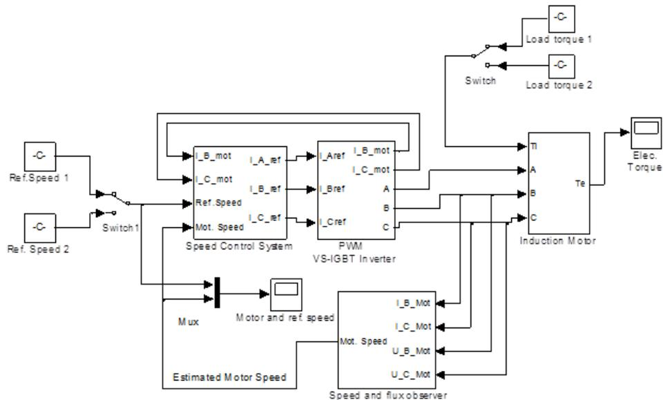
Figure 2. Simulink model of sensorless speed control system of induction motor
