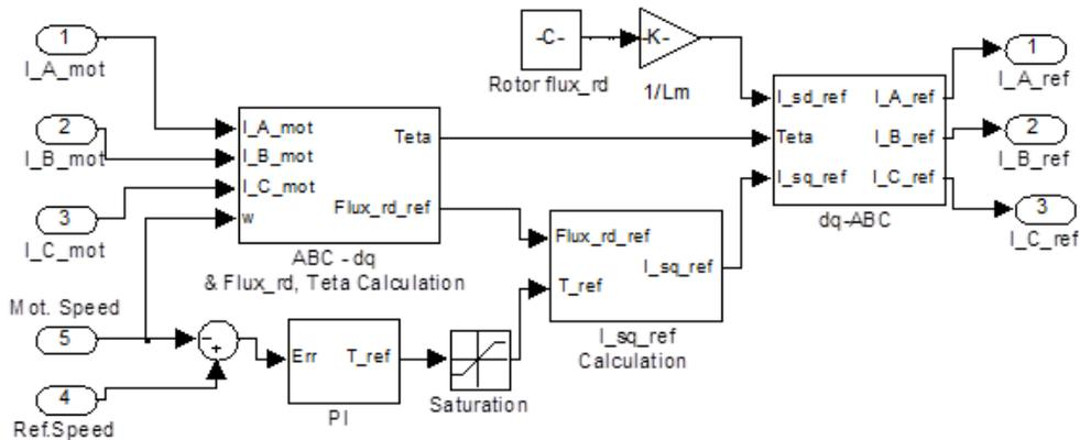
Figure 3. Simulink speed control system
