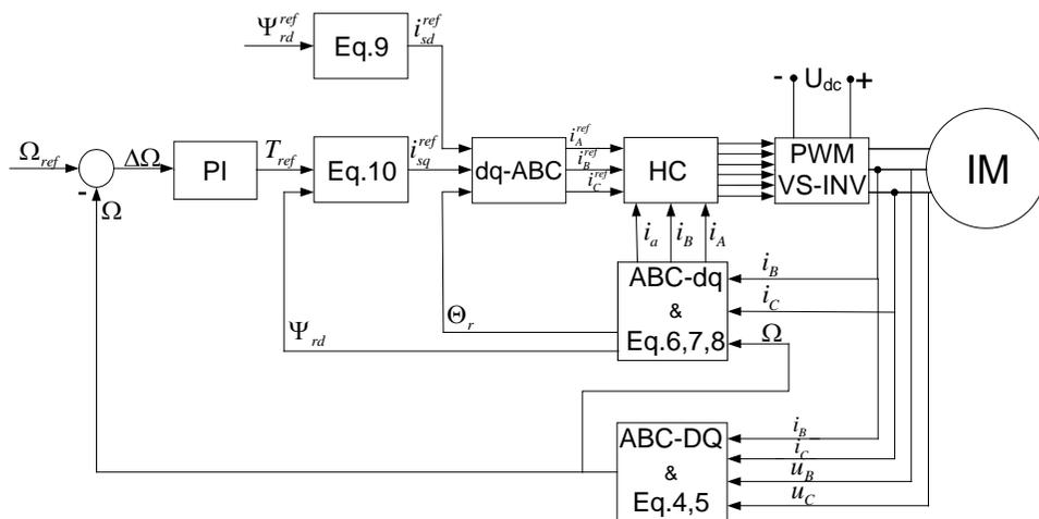
Figure 1. Sensorless speed rotor flux oriented control system of induction motor
