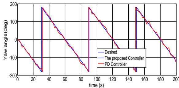
Fig. 5. Yaw angle tracking curves with sawtooth-wave command signal
