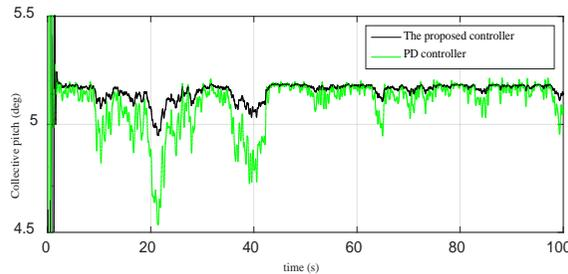
Fig. 4. Control input of vertical dynamics
