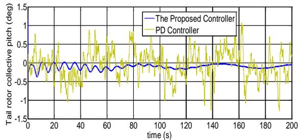
Fig. 8. Control input of yaw dynamics of an UAH
