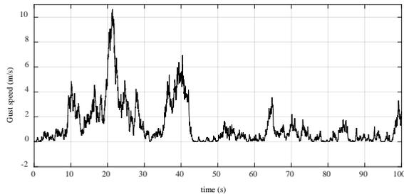
Fig. 9. Wind disturbance to test the controller
