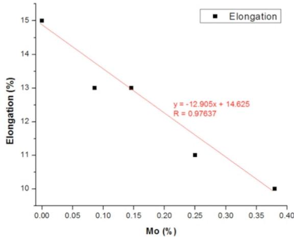
Figure 11. Molybdenum’s effect on the Ductility of Nodular Iron under Normal Casting Conditions
