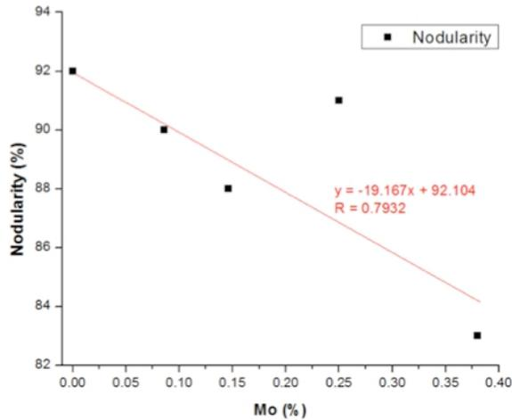
Figure 2. Effect of Molybdenum over the Nodularity under Nodular Iron Casting Conditions
