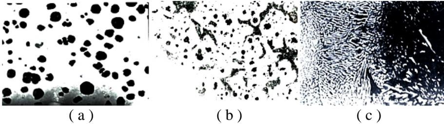
Figure 9. Photomicrographs of Nodular Iron with 0.250 % Molybdenum: (a) under normal casting conditions x 100, (b) attacked with 2 % Nital x 100, (c) interlamellar spacing of pearlite x 40,000
