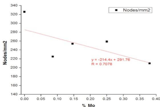
Figure 1. Effect of Molybdenum on the Number of Nodes in Nodular Iron Casting Conditions
