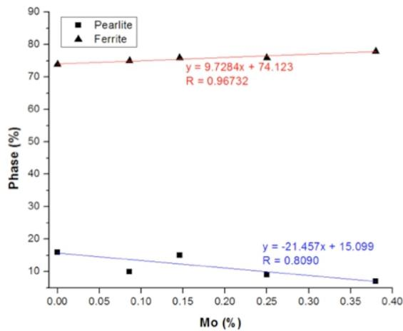
Figure 3. Effect of Molybdenum on the amount of Ferrite and Pearlite in Nodular Iron under Casting Conditions
