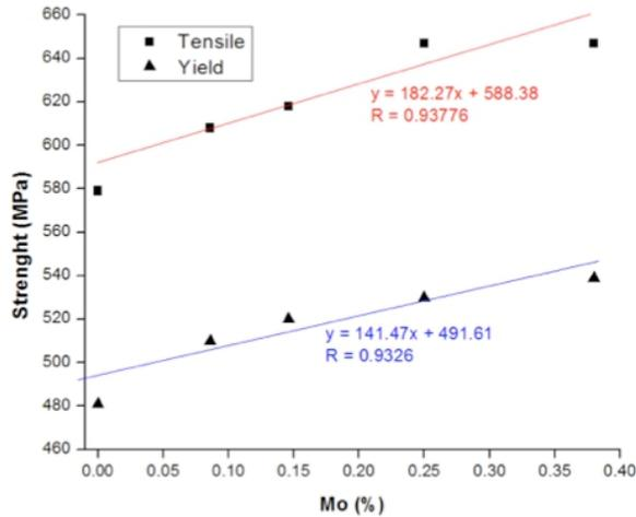
Figure 4. Effect of Molybdenum on the Tensile Strength and Yield Strength in Nodular Iron under Casting Conditions
