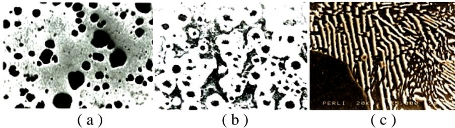
Figure 10. Photomicrographs of Nodular Iron with 0.380 % Molybdenum: (a) under normal casting conditions x 100, (b) attacked with 2 % Nital x 100, (c) interlamellar spacing of pearlite x 40,000
