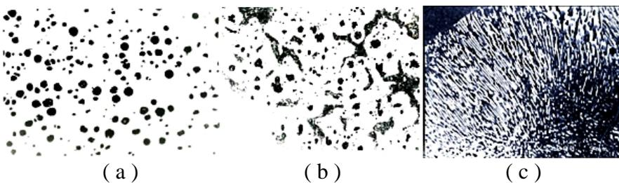
Figure 8. Photomicrographs of Nodular Iron with 0.146 % Molybdenum: (a) under normal casting conditions x 100, (b) attacked with 2 % Nital x 100, (c) interlamellar spacing of pearlite x 40,000
