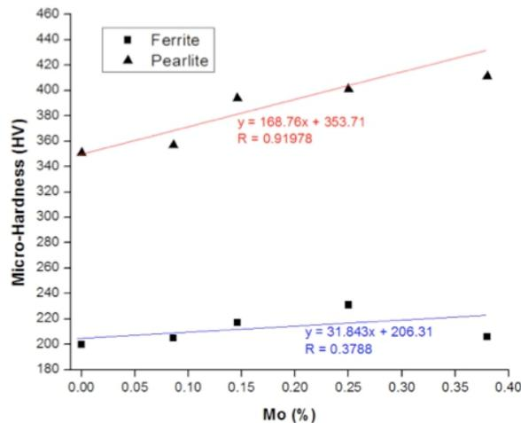
Figure 5. Effect of the Hardness of Ferrite and Pearlite according to the percentage of Molybdenum present in Nodular Iron under Casting Conditions
