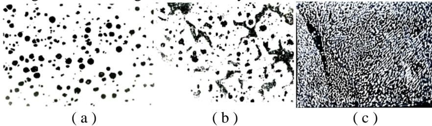
Figure 7. Photomicrographs of Nodular Iron with 0.086 % Molybdenum: (a) under normal casting conditions x 100, (b) attacked with 2 % Nital x 100, (c) interlamellar spacing of pearlite x 40,000
