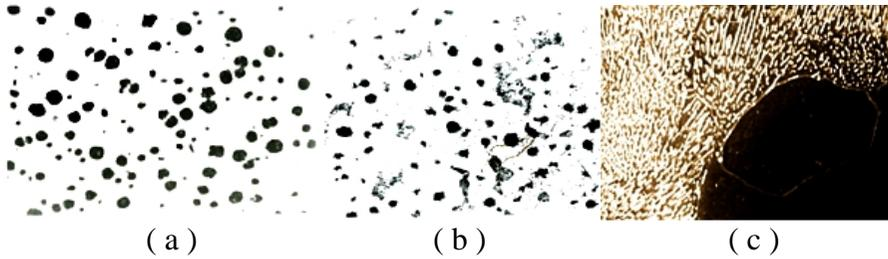
Figure 6. Photomicrographs of Nodular Iron without Molybdenum: (a) normal casting conditions x 100; (b) attacked with 2 % Nital x 100; and (c) interlayer spacing of the pearlite x 40,000
