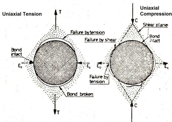
**Fig. 3:** Stress and strain state around a grain of aggregate<sup>27</sup>.
