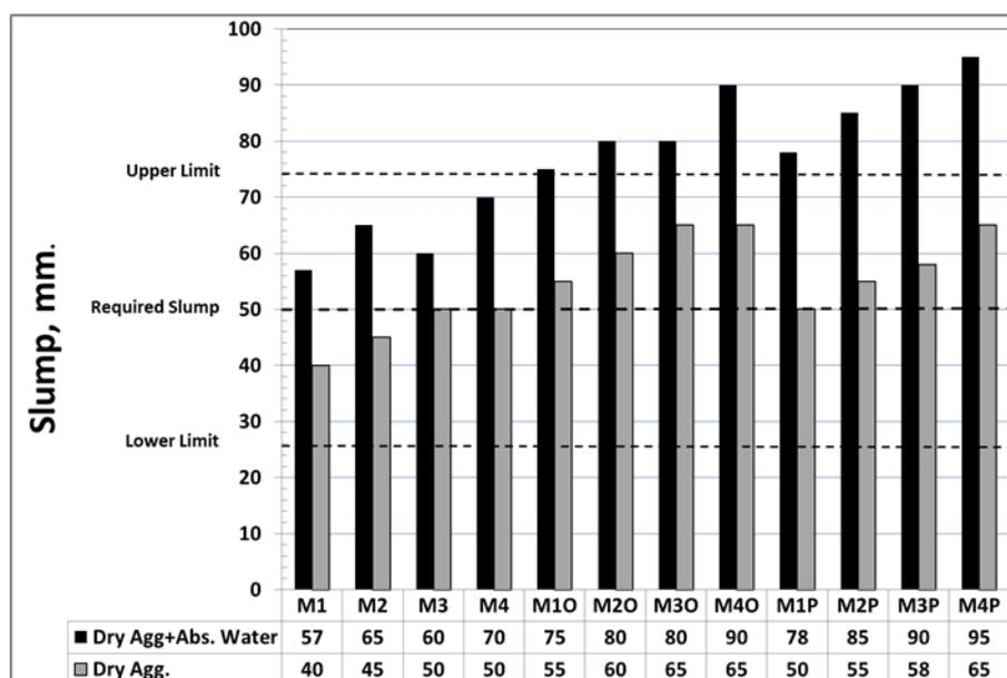
Fig. 5: Slump test results.
