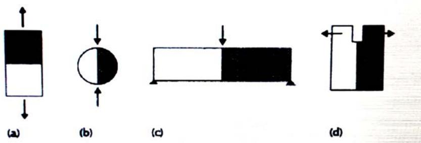
**Fig. 1:** Different composite test geometries for measuring the tensile or flexural bond strength between aggregate and cement matrix: (a) uniaxial tension test, (b) splitting tensile test, (c) three point bend test, and (d) wedge splitting test<sup>24</sup>.
