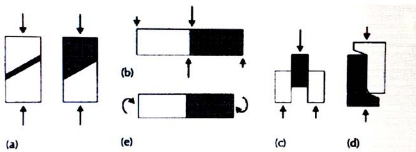
**Fig. 2:** Different composite test geometries for determining of the shear strength of the ITZ: (a) slant shear test, (b) four-point-shear beam, (c) push-through cube, (d) compact shear specimen, and (e) cylinder subjected to torsion [3].
