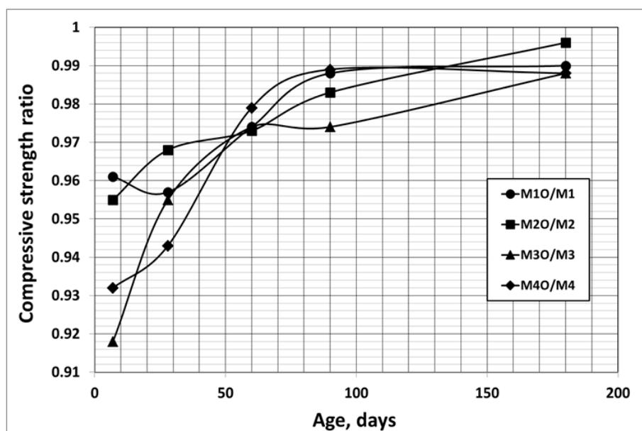
**Fig. 6:** The variation of compressive strength ratio with age for oil soaked aggregate mixes.
