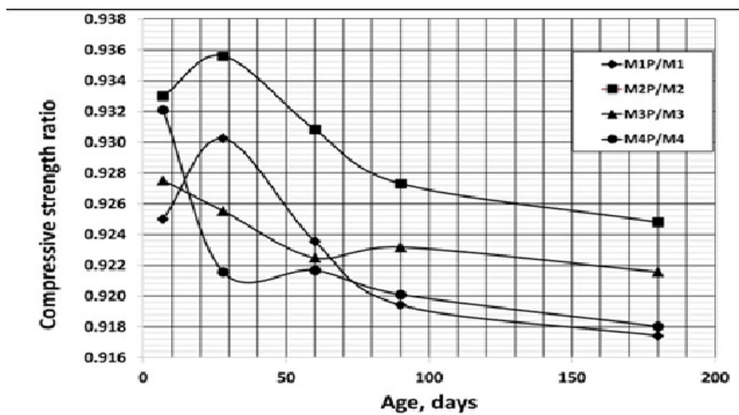
Fig. 7: The variation of compressive strength ratio with age for painted aggregate mixes.
