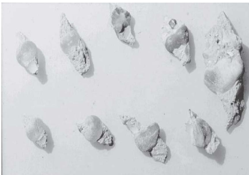
**Fig. 4:** Aggregate particles after failure in uniaxial compression<sup>31</sup>.
