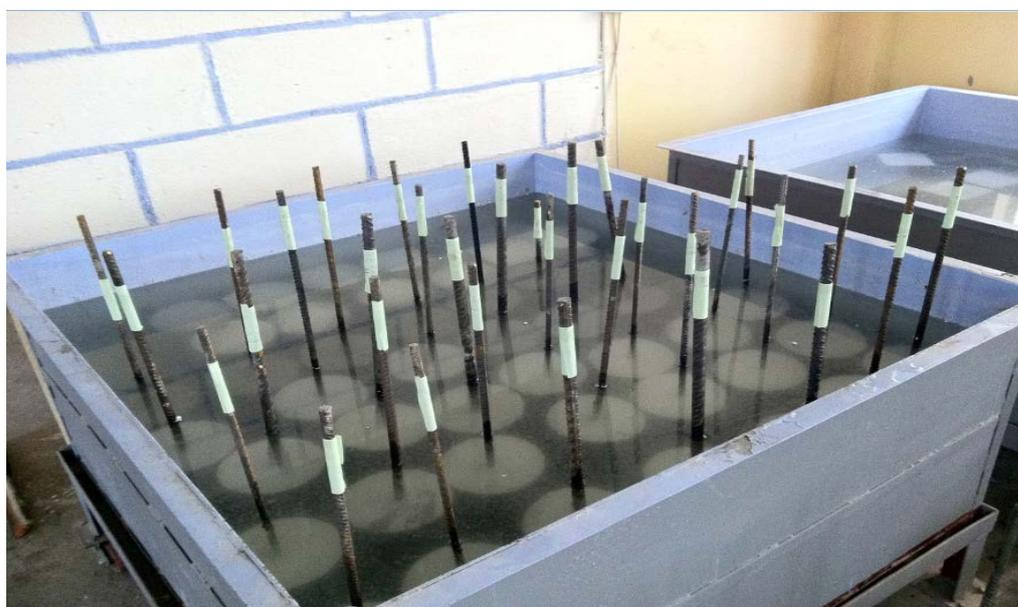
**Fig. 1b: Curing of the specimens**
