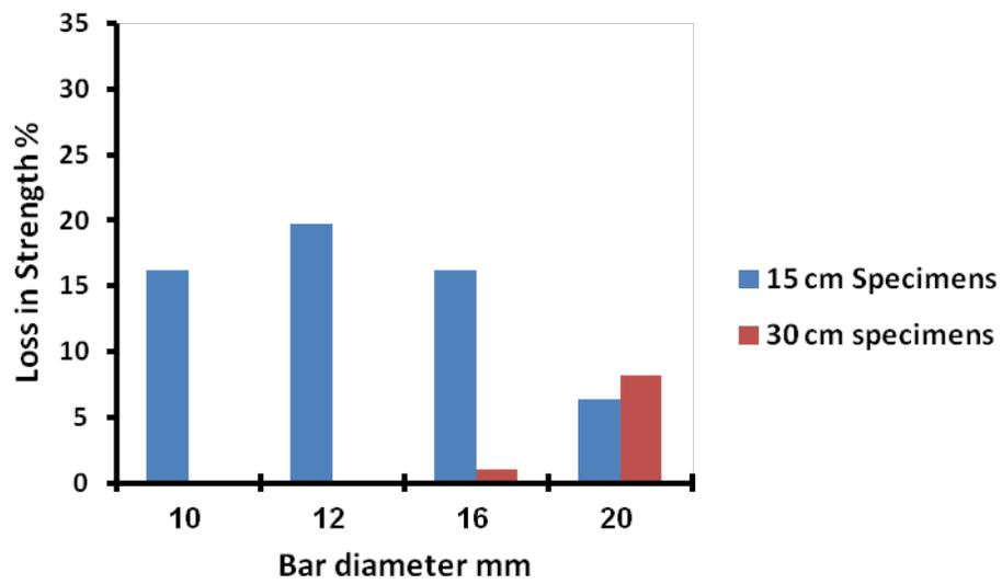
**Fig. 7: Average loss of bond strength due to 50% steel pollution**
