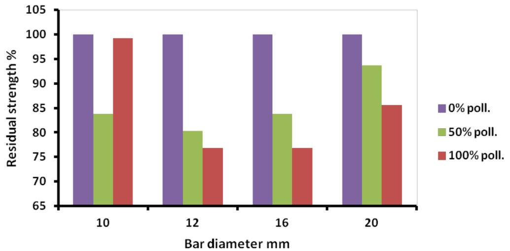
**Fig.10: Variation of residual bond strength with bar pollution for specimens of 15 cm length**
