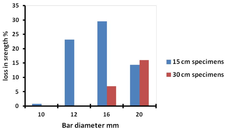
**Fig. 8: Average loss of bond strength due to 100% steel pollution**
