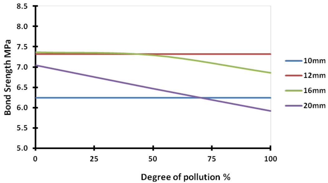
Fig. 5: Average bond strength of concrete with bars of 30 cm length
