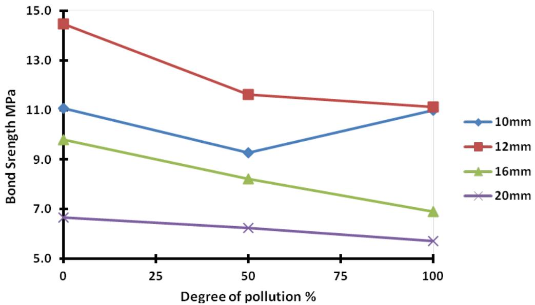
Fig. 6: Average bond strength of concrete with steel bars of 15 cm length
