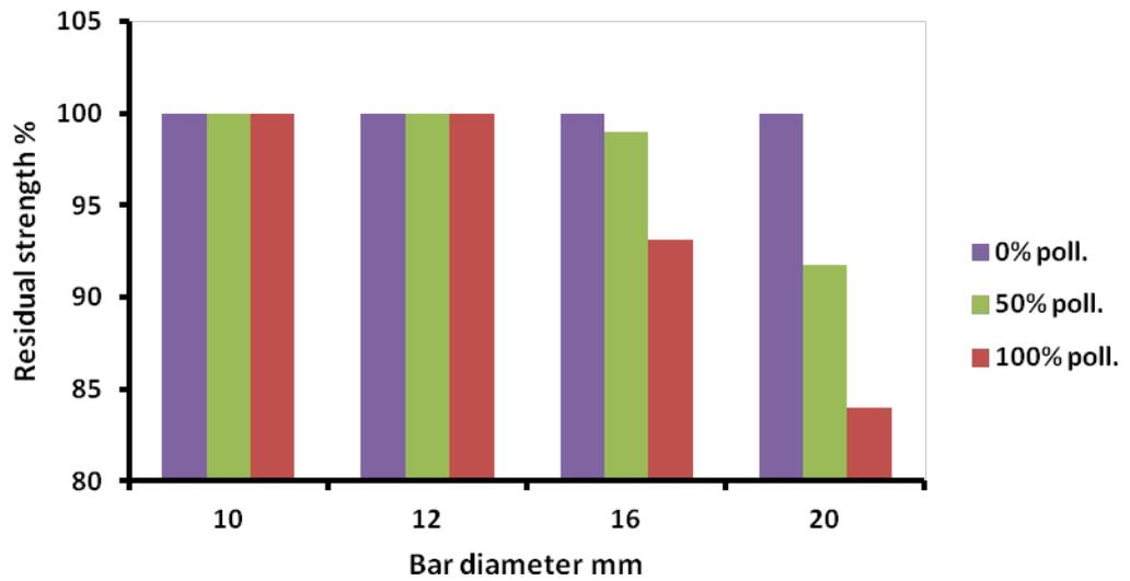
**Fig. 9: Variation of residual bond strength with bar pollution for specimens of 30 cm length**
