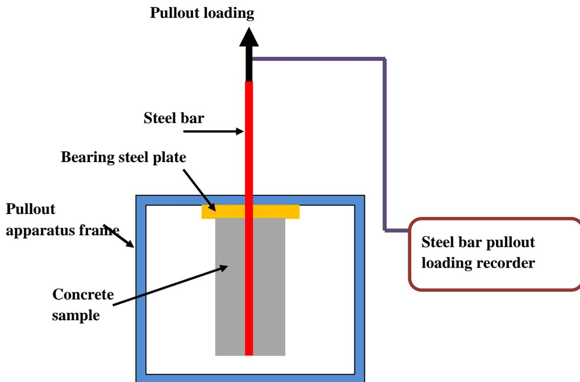
**Fig. 4: Schematic layout of present bond stress test**
