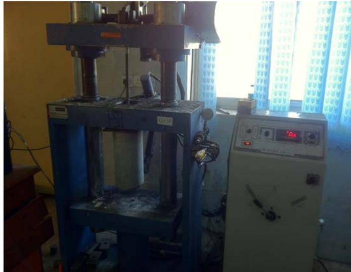
**Fig. 3: Pull-out test specimen and loading machine**
