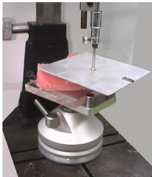
Figure 1. The apparatus used for parallelizing the base of the lower acrylic cast to the occlusal plane.
