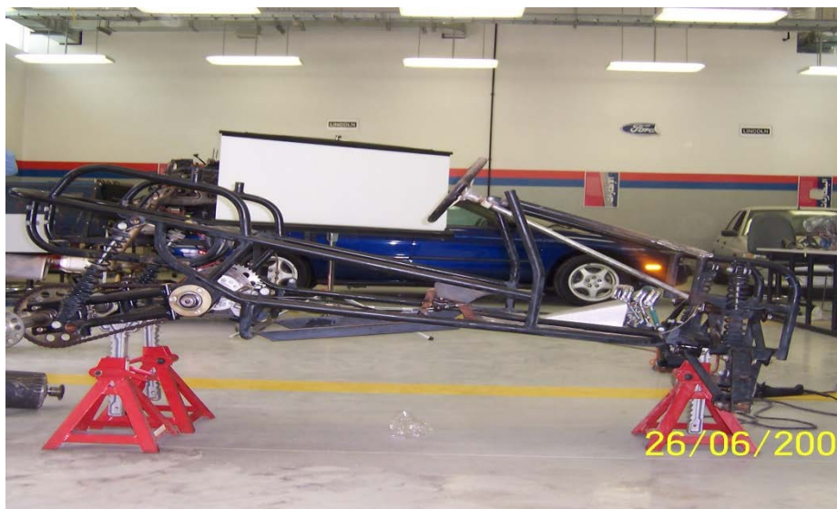
Fig. 5: Chassis, front and rear suspension
