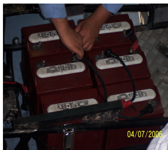
Fig. 9: Electric motor installation and aligning Fig. 10: Batteries connection and installation
