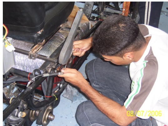
Fig. 17: Hand brake installation
