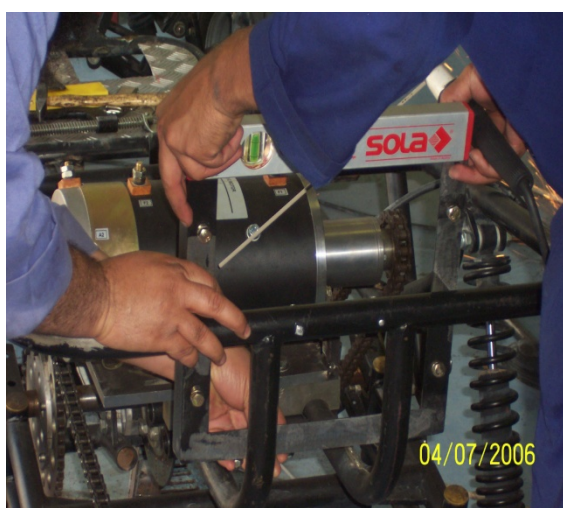
Fig. 9: Electric motor installation and aligning Fig. 10: Batteries connection and installation
