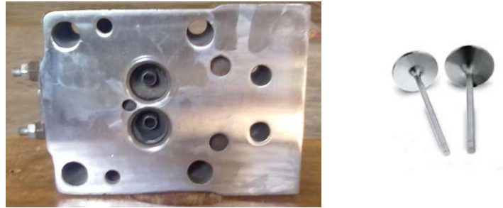
Figure 2: PSZ coated cylinder head and valves
