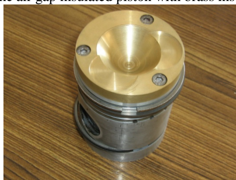
Figure1: An air-gap insulated piston with brass insert
