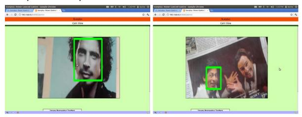
In the **Face Detection** mode, we process subsequent frames using the Android's camera. If and when a face is detected, a green box is drawn around the face on the output image. It is implemented using openCV and the LBP Cascade Classifier through XML in the Android application. The screenshots show that the Cascade Classifier does a good job of finding faces in an image, but as can be seen from the third image, it still is not perfect.
