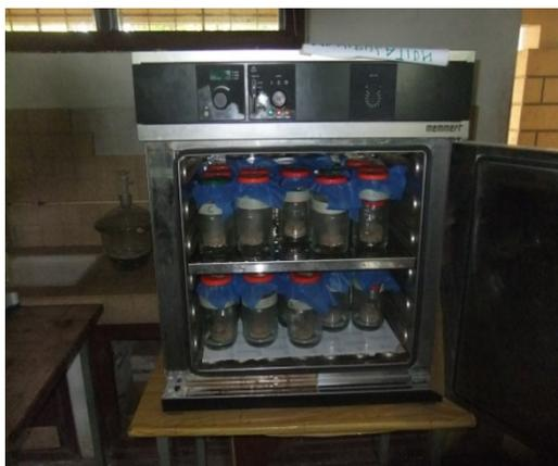
**Figure 2:** Experimental apparatus for desorption isotherms
