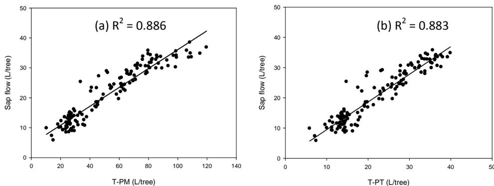
**Fig 2.** Relation between the measured sap flow rate and transpiration predicted by the PM equation (a) and by the PT equation (b).
