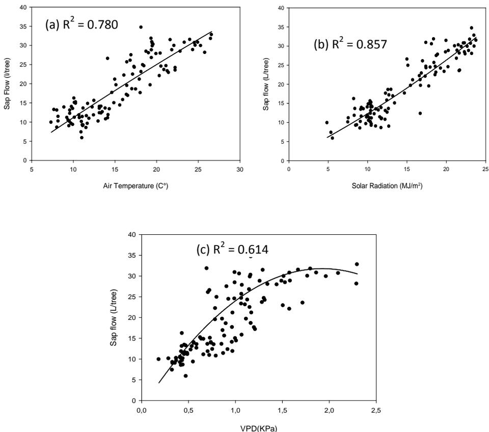
**Fig.1.** Relation between the daily measured sap flow rate and air temperature (a); solar radiation (b) and vapour pressure deficit (c)
