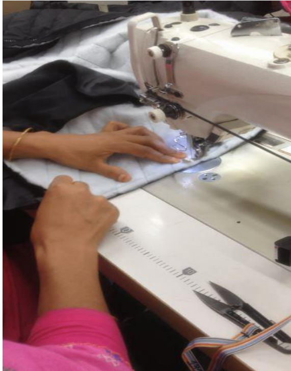
Figure 8. Shell lining join at center front
