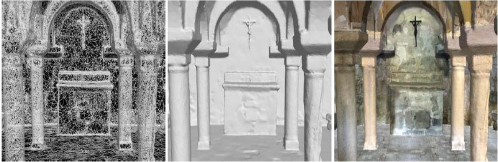
Figure 3: Different renderings (wireframe, shaded and textured mode) of a surveyed and modeled underground church. (Remondino, 2011).
