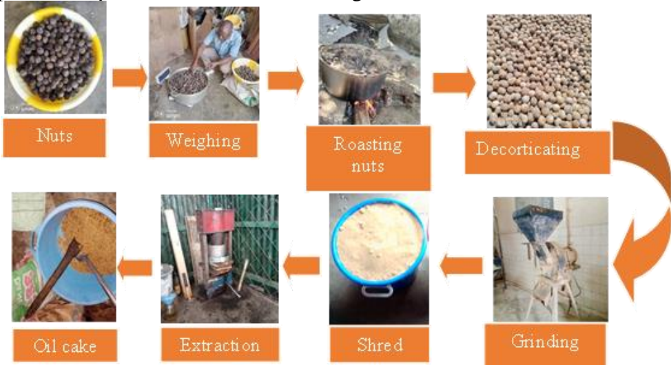
Figure 1: Production of T. conophorum oil cake
