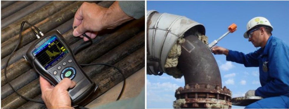
Photos 3: Measurement of the evolution of corrosion
